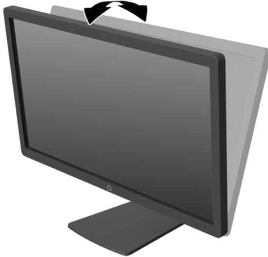
2. Swivel the monitor to the left or right for the best viewing angle.
