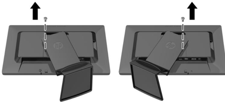
4. Rotate the base of the monitor up (1) then pull it back (2) to unhinge the tabs on the monitor stand from the slots in the monitor.
